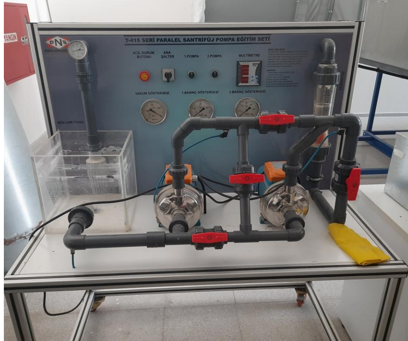
Fig 1. T-415 Serial/Parallel Centrifugal Pump Test Set
