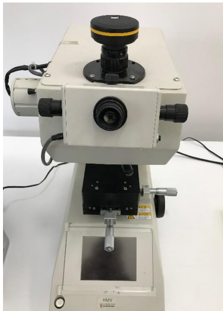
Figure 1: SHIMADZU HMV Microhardness Tester
