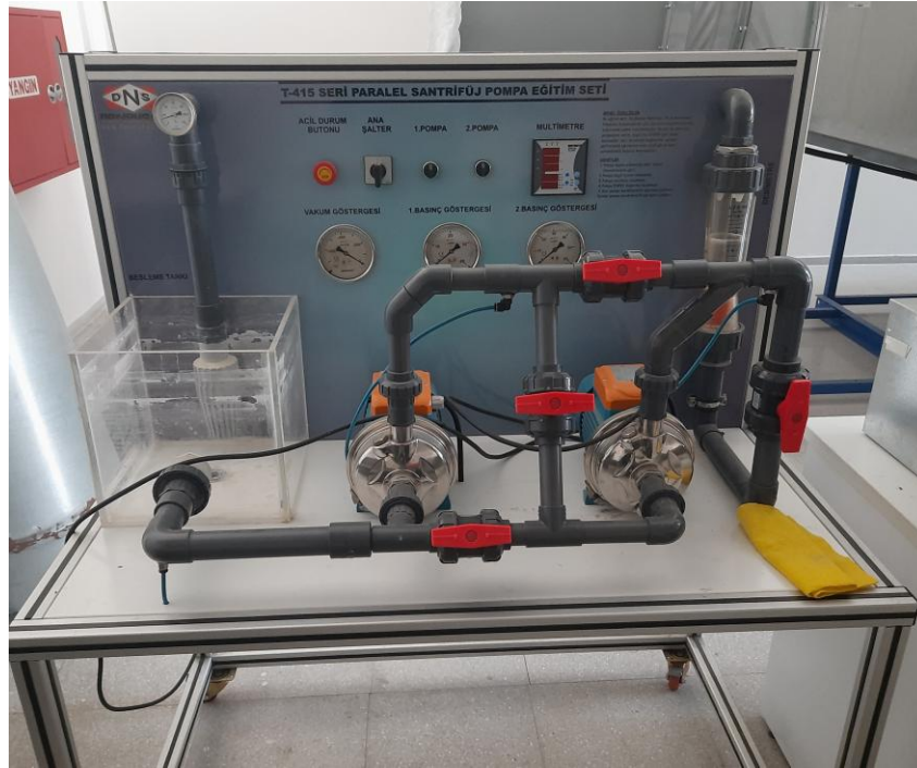
Fig 1. T-415 Serial/Parallel Centrifugal Pump Test Set
